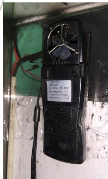
(c)排氣口風速量測
