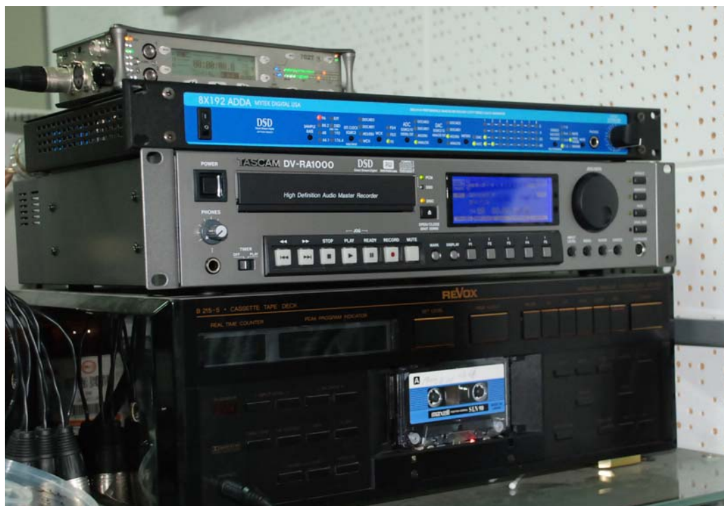
圖 4-2-3 由上而下的轉檔工具為 Sound Device 702T; A/D Converter; TASCAM DV-RA1000; Nakamichi Bx-2 Tape player
