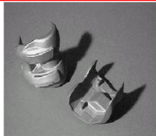
Photo 6. Example of two cobalt chrome knee implant investment castings (Biommet)
