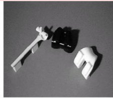
Photo 5. ABS IC pattern for an elbow (with galling) and two knees (Biommet)
