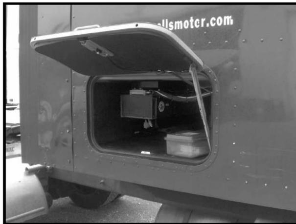
Figure 20. The Main DAS Unit Mounted in a Compartment Located on the Side of the Truck
