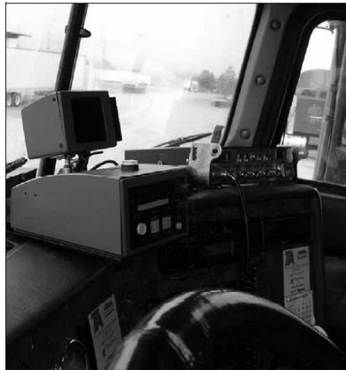
(b) Modified DFM position with bracket to get DFM closer to (in front of) driver
